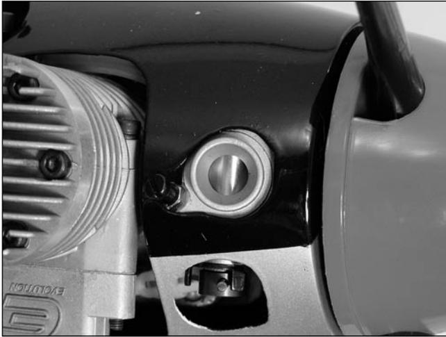
Move the trim lever up towards the top of the transmitter. The barrel in the carburetor should have an opening of around 1/16".
